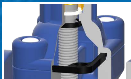
Round rubber gasket on recess in bonnet prevent blow out by pressure surges (Gate valve)
