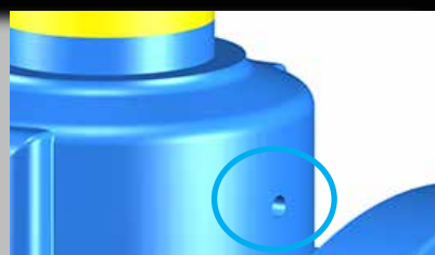
Witness hole to detect leakage at diaphragm failure
