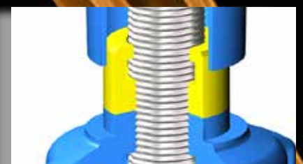
Grease reservoir integrated in the spindle chamber that lubricates the spindle along operations thus avoiding valve spindle jamming
