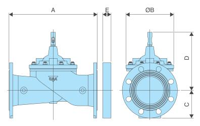
The dimension E in the picture above refers only to applications where it is necessary to add a flanged orifice downstream or upstream of the valve, for example for flow control or cavitation prevention.
