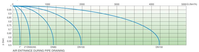
The air flow charts were created in Kg/s from laboratory tests and numerical analysis, then converted in Nm<sup>3</sup>/h using a safety factor.
