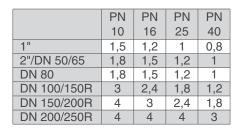
Nozzle diameter in mm according to the size of the air valve and the PN.
