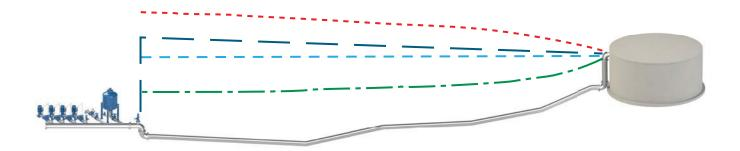
The plot above shows the pressure envelope of the transient event caused by pump failure on a pipeline with A.V.A.S.T. installed as a protection. The red and green are the maximum and minimum pressure values reached during the simulation, it is clearly visible the beneficial effect in terms of negative pressure and consequently reduction of water hammer.
