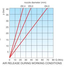
The air flow charts were created in Kg/s from laboratory tests and numerical analysis, then converted in Nm³/h using a safety factor.
