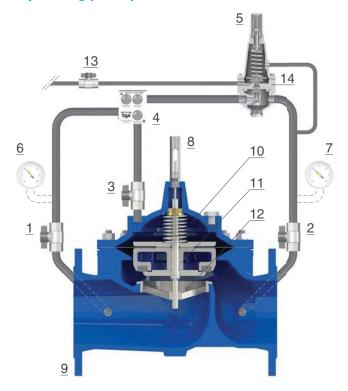
The CSA Model XLC 495 is operated by a two ways pilot (5), with pre-set and adjustable set point value, sensing two pressures points in order to maintain a required differential between them.
