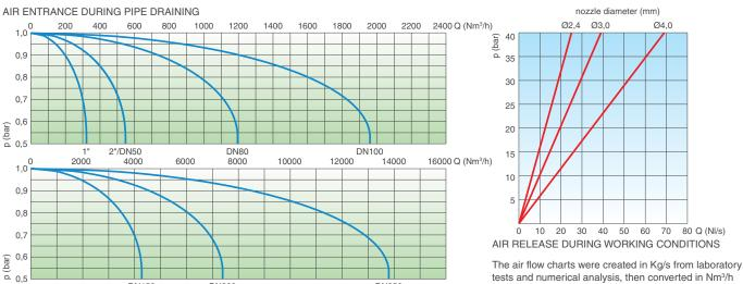
tests and numerical analysis, then converted in Nm3/h DN150 DN200 DN250 using a safety factor. AIR ENTRANCE DURING PIPE DRAINING
