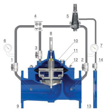
The CSA model XLC 430 is operated by a two 2 ways pilot (5), for flow control, with pre-set set and adjustable values, sensing the drop in pressure produced by the orifice plate (13), where a stainless steel disk is inserted inside a flange and connected to the pilot with a sensing line (14) non supplied.
