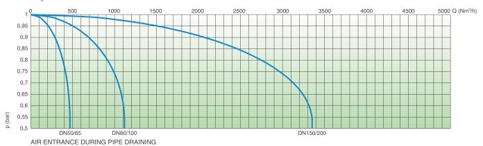
The air flow charts were created in Kg/s from laboratory tests and numerical analysis, then converted in Nm³/h using a safety factor.
