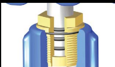
Triple O-ring stem sealing (Gate valve)
