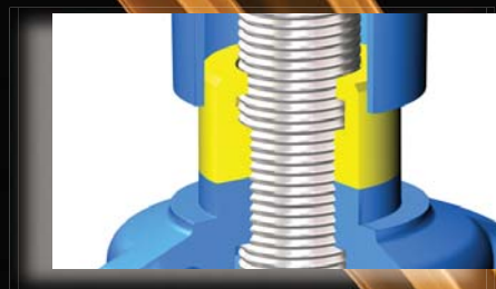
Grease reservoir integrated in the spindle chamber that lubricates the spindle along operations thus avoiding valve spindle jamming
